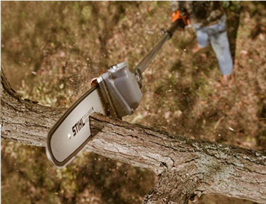
Figure 3 Clean Cut by motorized pruner
